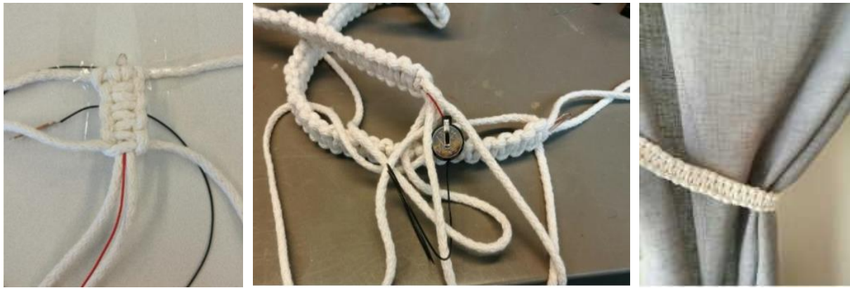
FIGURE 2. From left to right: An electric wire runs inside the fastener that is made using a macramé technique. A 3-volt battery is used as a power supply and the wires are soldered as a circuit. No board is included, but the LED, battery and wires are used. Normally, when privacy is not needed, the fastener simply keeps the room divider open between the spaces. A small press stud acts as a switch and an LED light is placed at the end of the fastener (left side, not visible in the picture). The light goes on when the switch is pressed. This indicates a reserved space when more privacy is needed. Images: Iina Mähönen.
