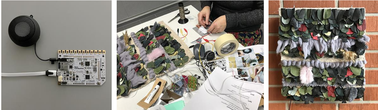
FIGURE 4. From left to right: A Bare Conductive Touch Board plays sounds and voices when touched. A student exploring textile materials and technology in the workshop where the participants were provided with Bare Conductive boards and a variety of electronic tools, soft design materials (e.g., felt, fur, fabrics), and various wiring components (conductive thread, conductive ink, copper tapes, crocodile clips, tin foil). The finalised work in the exhibition is called “Come Well”, an e-textile containing an embedded touch board. Images: Emmi Harjuniemi.
