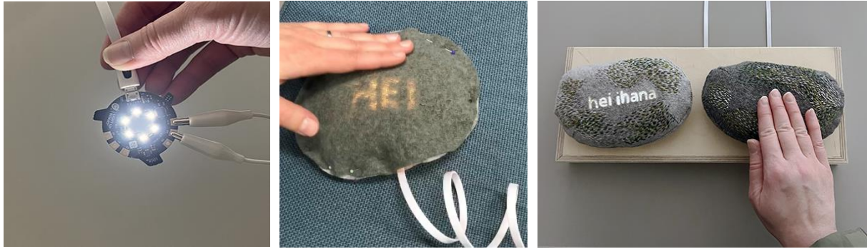
FIGURE 3. From left to right: Testing the Light Up Board’s settings of the six built-in-LEDs by connecting electrodes differently. The student’s first rapid prototype made in the workshop. Finalized artwork of the “Secret Message”, an e-textile product where text is lighted with the integrated LEDs in the Light Up Board. Images: Emmi Harjuniemi.
